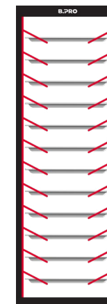
12 supports each with 100 mm spacing
